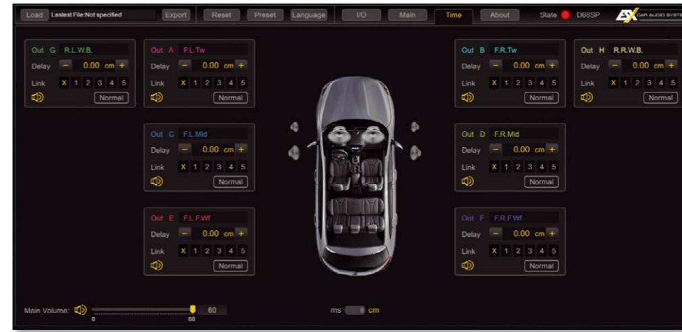
Here the delay time of the outputs is adjusted. The loudspeakers are placed nicely in the car – here Mercedes with footwell woofers
