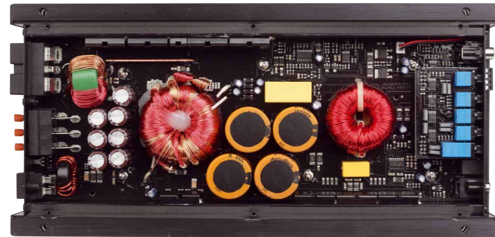
The M FOUR DSP, on the contrary, works with two small amplifier ICs
