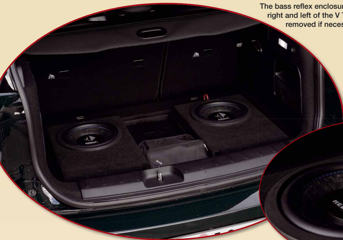
Two 10-inch helix K 10W subwoofers are responsible for the low bass. The 2 x 2 Ohm dual voice coils harmonize beautifully with the V TWELVE DSP
