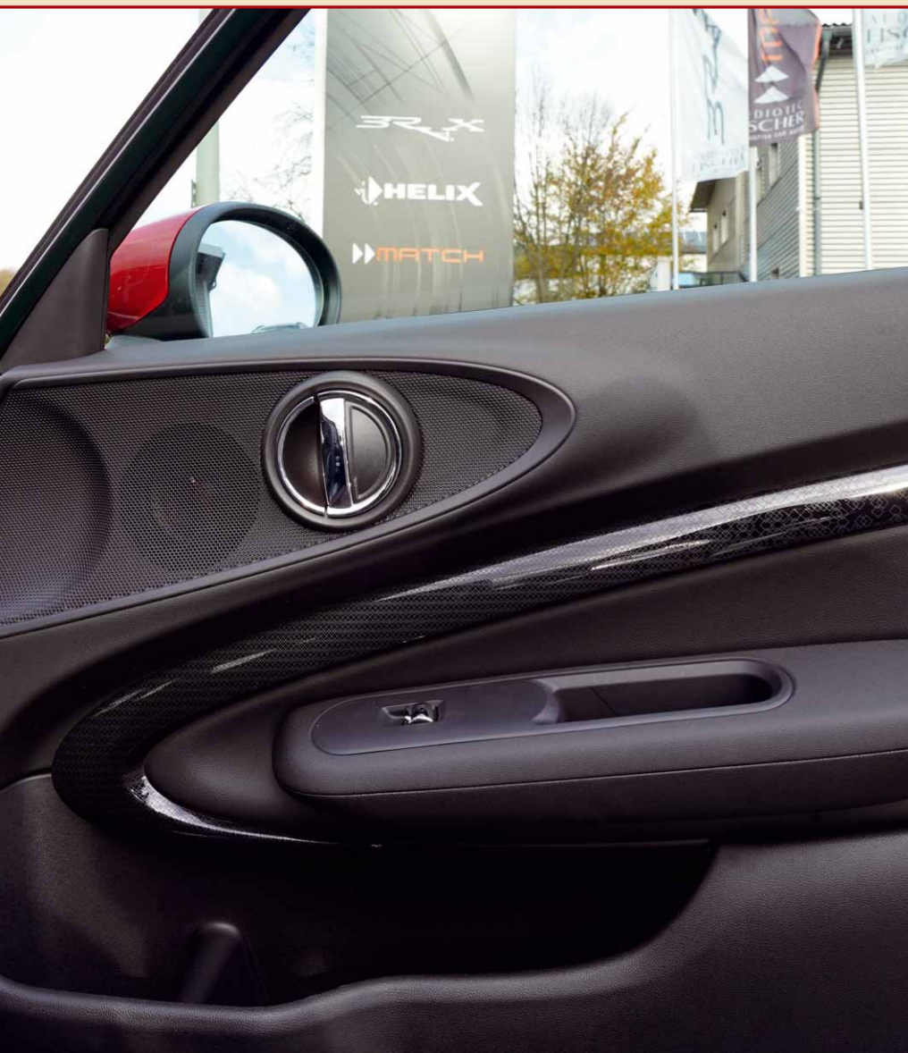
Originally there are only broadbands in the doors. The Match loudspeakers for BMW are suitable for Mini as well
