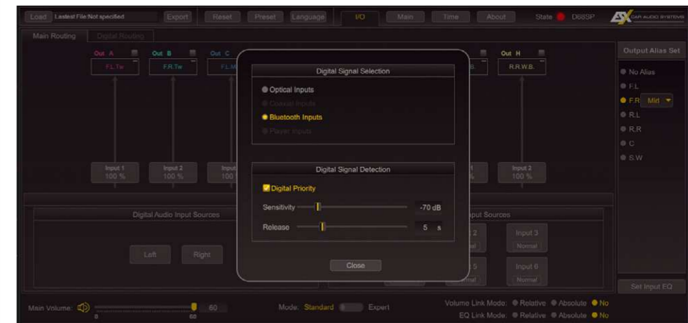
The digital inputs can be prioritized so that they are switched over when a signal is received. Here Bluetooth gets priority; after 5 seconds of silence, it will be switched back to analog
