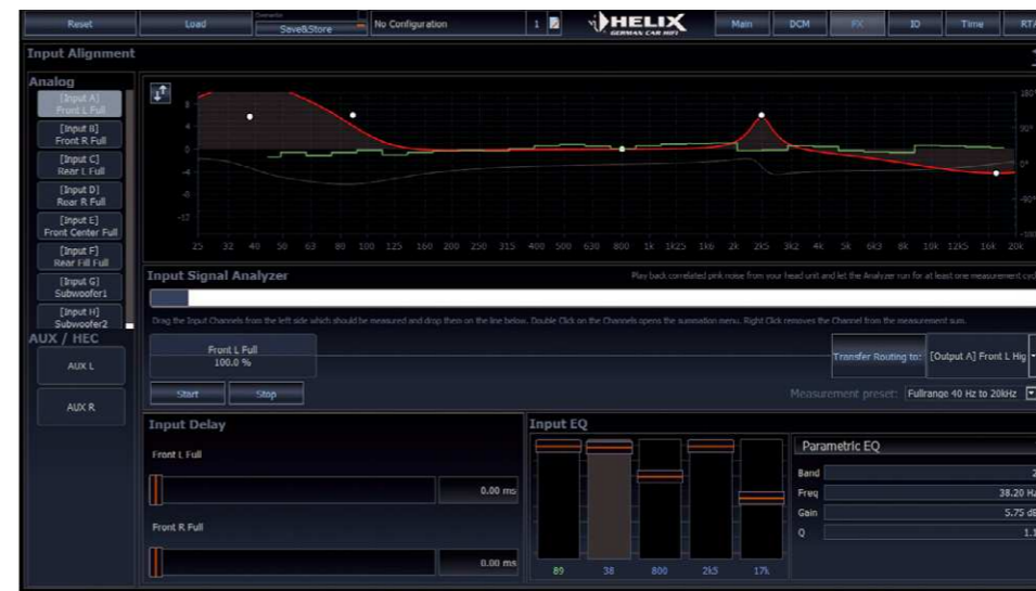
In the ISA, any inputs and their sums can be measured. EQ (with allpass) and time alignment are adjusting the incoming signal
