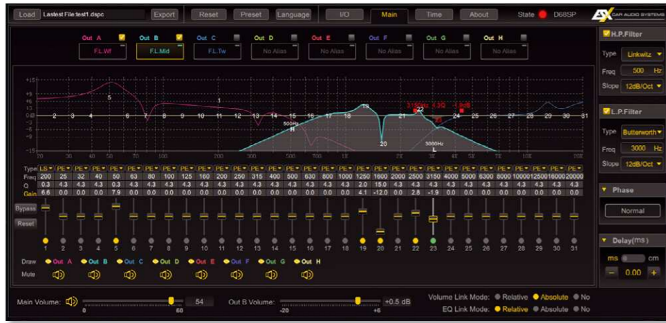
Equalizers and crossovers are set on the main screen. Master and channel levels are available, and absolute or relative linking of channels is possible
