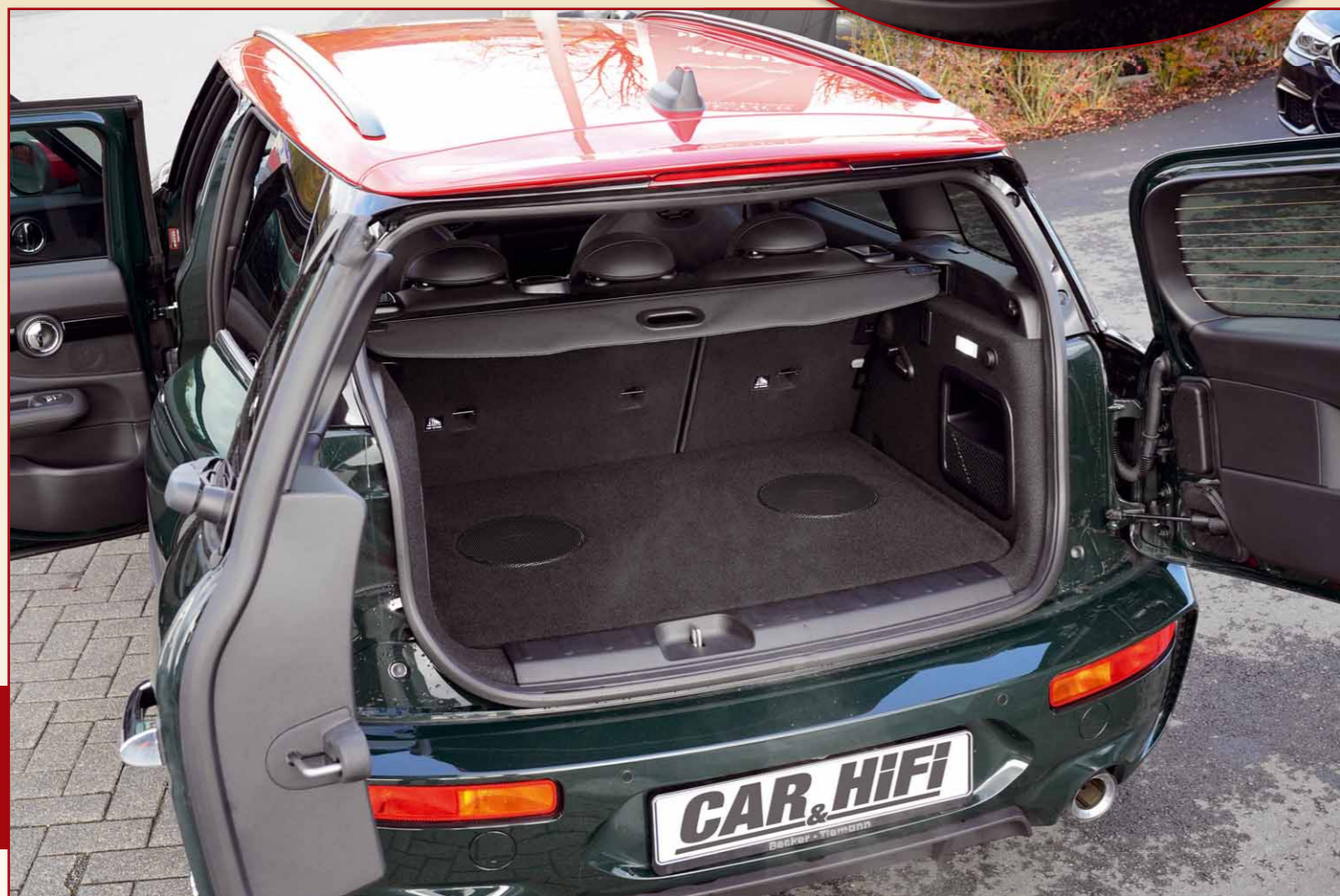
Of course, the Clubman trunk remains fully usable. There are a power amplifier and two bass cases under the floor.
