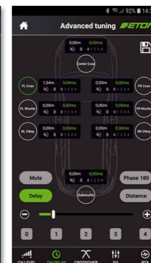
In the runtime menu, there are also buttons to reverse polarity and mute individual speakers
