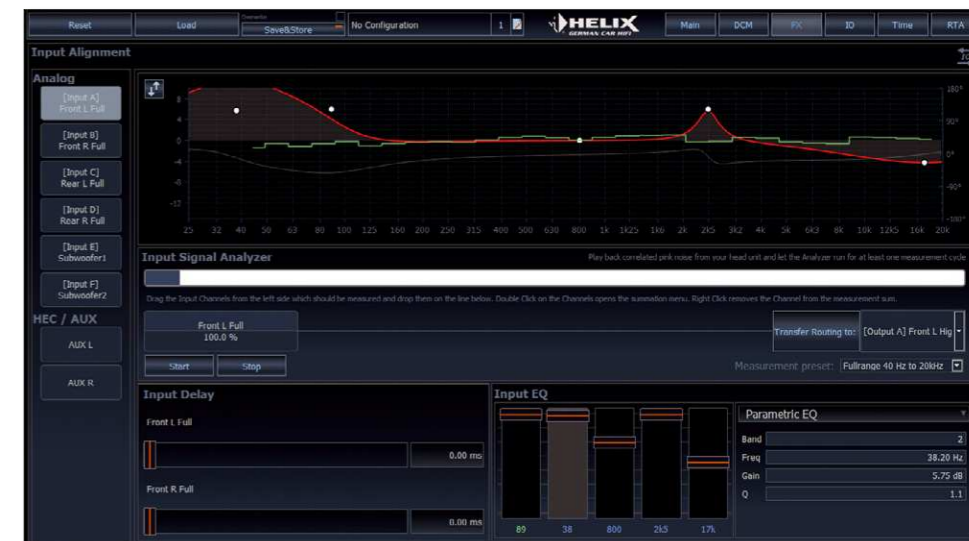
In the ISA, any inputs and their sums can be measured. EQ (with allpass) and time alignment are adjusting the incoming signal
