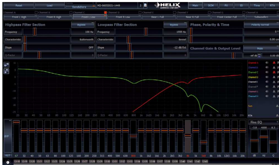
With the HEC BT HD, the PC software DSP PC-Tool can now also be used for wireless programming
