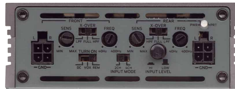
The fronts of the A-series measure only 105 x 40 mm. The signal input is via Molex connectors, either higher low-level
