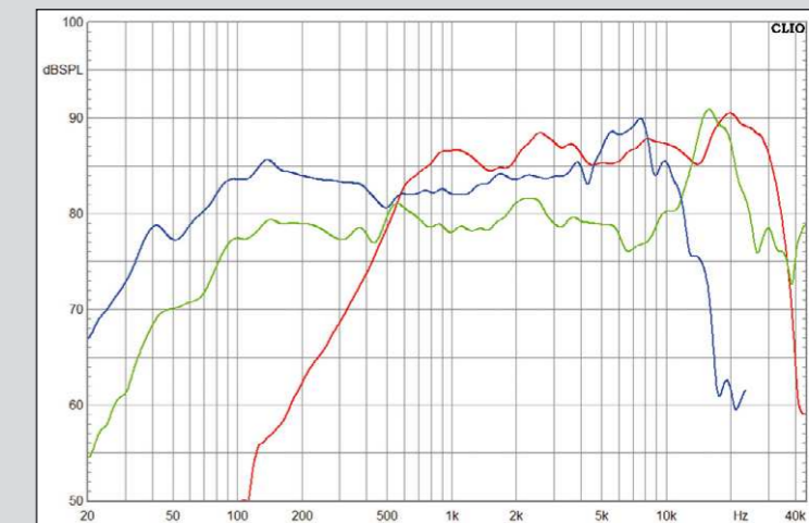
Already the woofer and the tweeter show a wide common frequency range. The midrange driver can be decoupled from 150 Hz with any crossover frequency.
