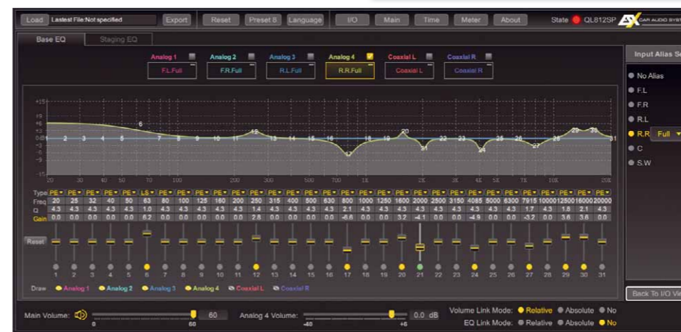
In addition to the input EQ, there is a staging EQ with 31 bands per channel as well
