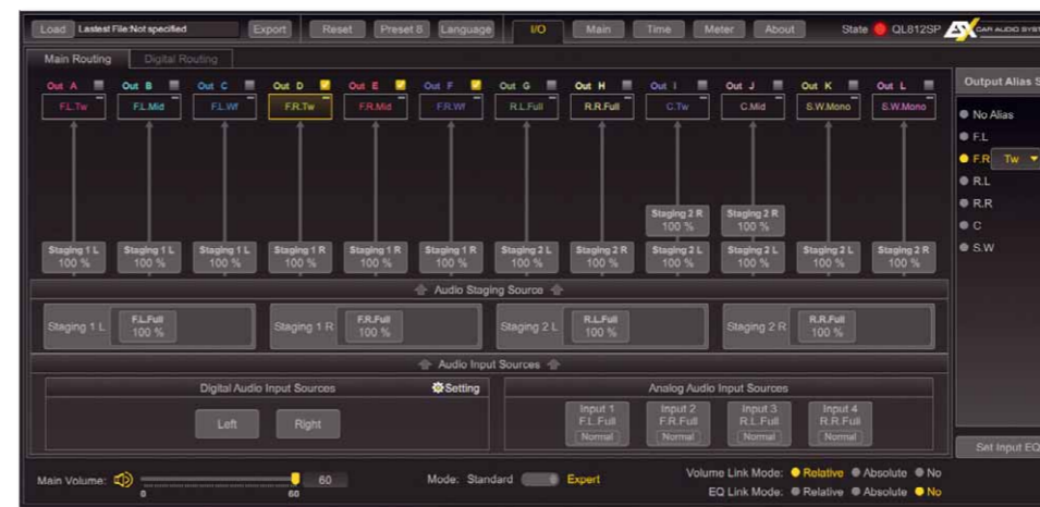
In expert mode, a new staging channel with a dedicated EQ emerges between inputs and outputs
