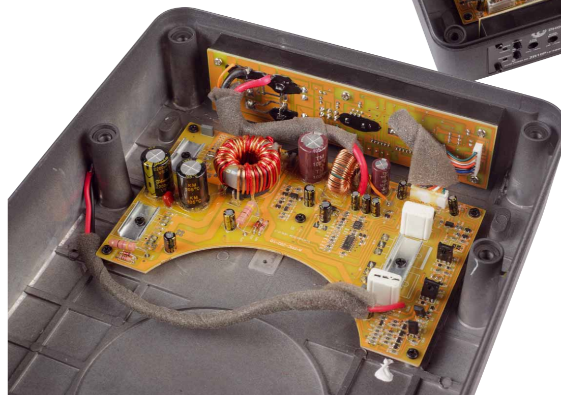
The amplifier is a well known class AB design, but it provides more than enough power
