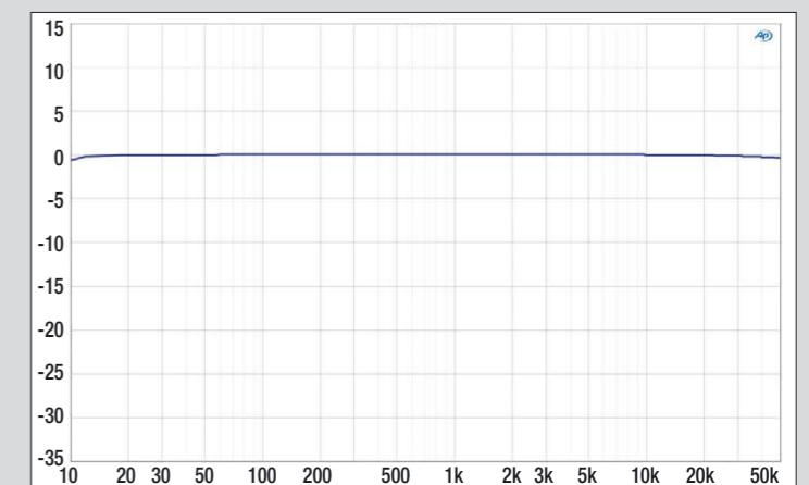
After spreading the Y-axis, a minimal drop of 0.7 dB can be seen at the edges. The A-2 works very broadband and linear
