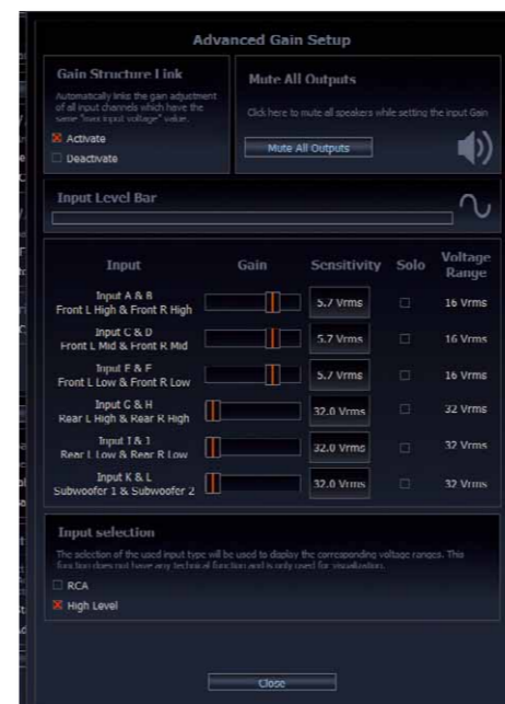
In the advanced gain set-up, the sensitivity of the inputs can be adjusted separately; the maximum possible is automatically detected and the current input level is displayed along with a clipping warning
