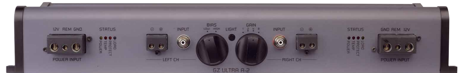
First class wire terminals and RCA sockets and four status LEDs are nice, but mainly the two switches catch the eye
