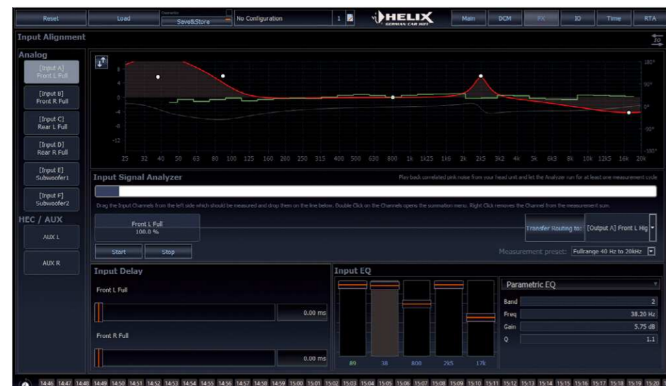
In the ISA (input stage analyzer), the inputs can be measured and directly corrected by time and equalizer
