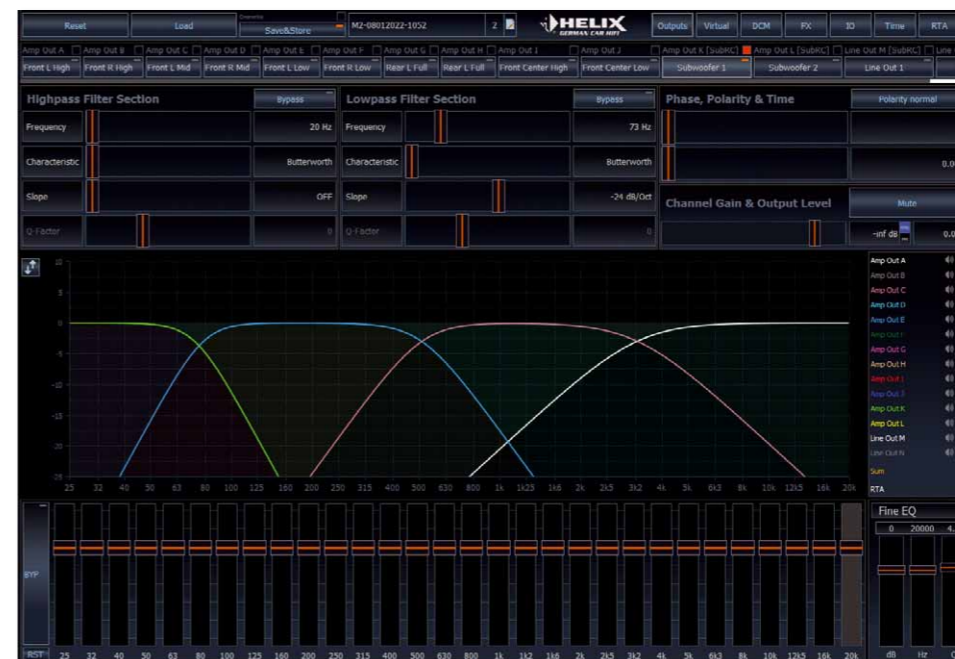
The twelve output channels just fit next to each other. Bandpass crossovers, 31 EQ bands, phase and time and channel level are each available per channel
