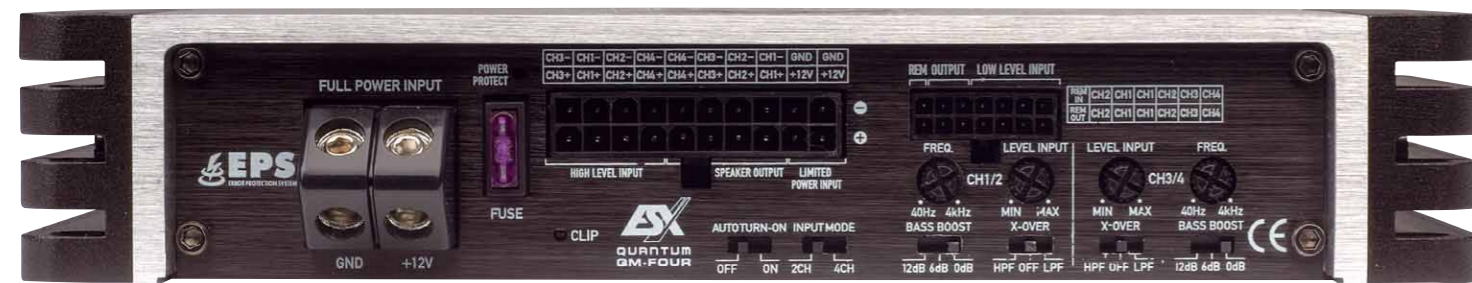
All signal and speaker connections are bundled in two Molex connectors
