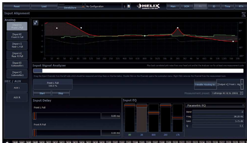
The ISA (Input Stage Analyzer) features single or combined measurement of the input channels. Time alignment and equalizing can be applied immediately
