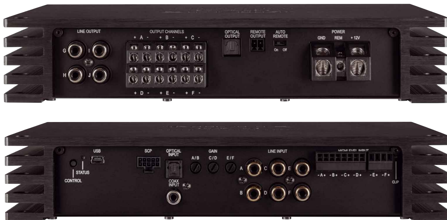
The 6 processed outputs are distributed over 4 RCA sockets and the digital optical output. The inputs feature 6 x RCA, 6 x high-in and digital, either optical or coax
