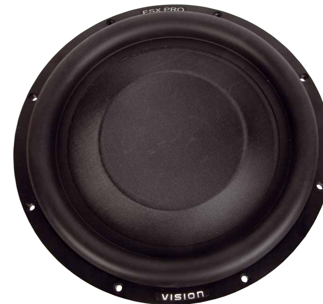
The surrounds are narrow to maximize the cone area, but the high profile still allows for large excursions
