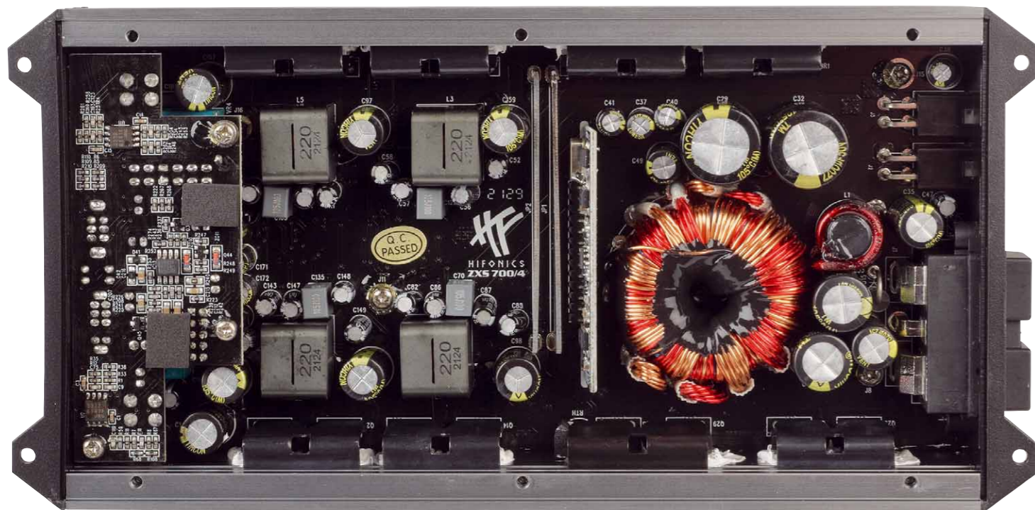
Modern, highly integrated design: 4-channel amplifier with large power supply (left) and Class-D inductors with outer magnetic capsules
