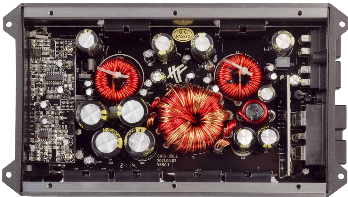
Modern, highly integrated design: 2-channel amplifier with large transformer for power supply and two Class-D inductors
