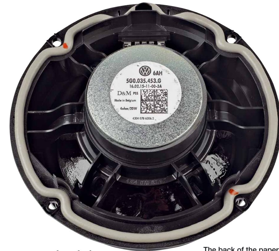
The back of the paper cone also receives a stiffening coating
