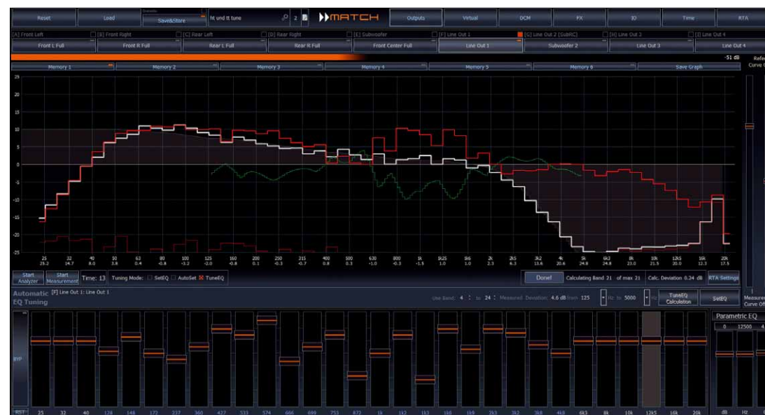
RTA measurement of a mid-range woofer: Original curve (red) and result with 24-dB crossing (white). You can see the correction via TuneEQ in green and, at the bottom, the EQ bands 4 – 24 are accordingly adjusted. We measured with an accuracy of 1/6 octave and standard smoothing; finer is possible if desired
