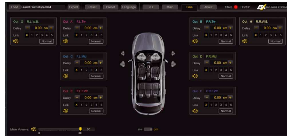
Here the output time alignment is set. The speakers are displayed nicely in the vehicle. Here, we see a Mercedes with footwell woofers as an example
