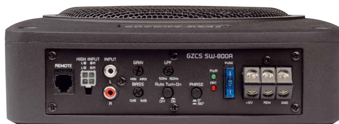
Speaker-level inputs are available as well as a polarity switch, a low-pass filter, and a bass boost
