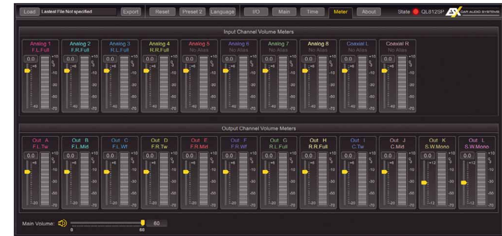
The SPL of all eight analog inputs and 12 outputs is displayed and directly adjusted
