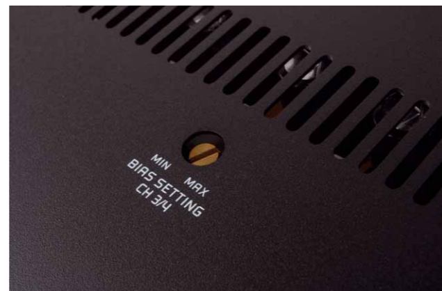
For circuitry reasons, the bias potentiometers are located at the bottom of the cabinet; there is one per channel pair
