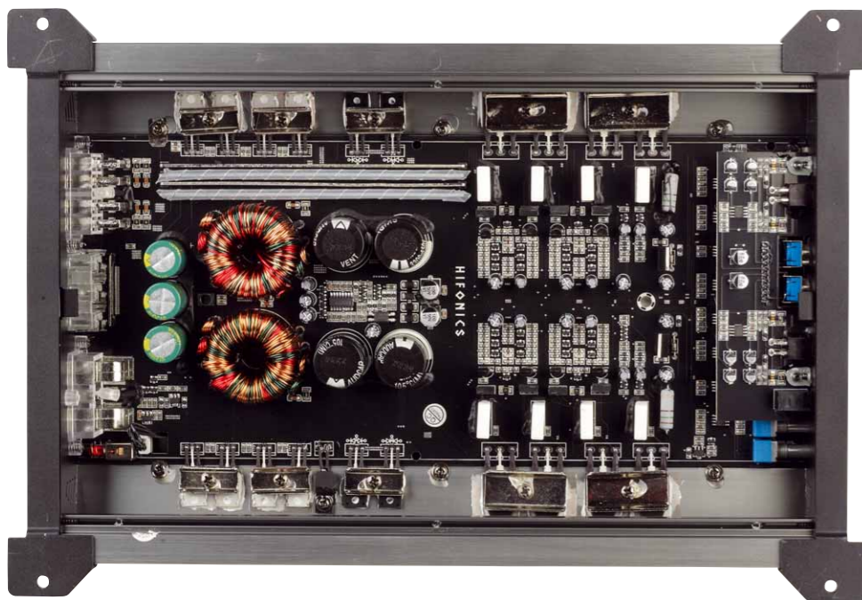
The four-channel amp features an , analog' class AB board
